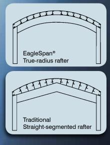
The true curve of EagleSpan<sup>®</sup> (top diagram) offers three key advantages over straight rafters with graduated length purlin clips (bottom diagram): the lower cost of uniform clips, a broad range on the radius of the curve, and the congruence of an interior curve to maintain consistency with the exterior.
