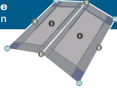
Standard industry wind tunnel tests on various roof configurations have shown that the wind loading on a roof is divided into three zones:
