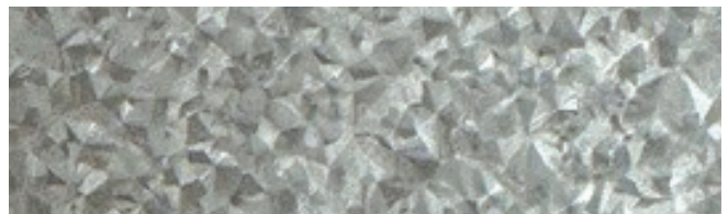
Galvalume (GL) This provides weather protection. It is not intended as a uniform finish. Natural variations in appearance are normal. (Not Painted)
